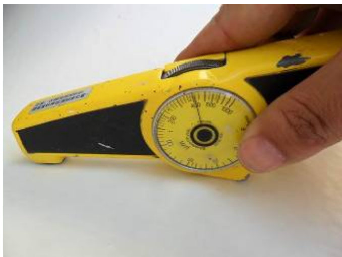
37. Epoxy resin paint thickness : 410µm
