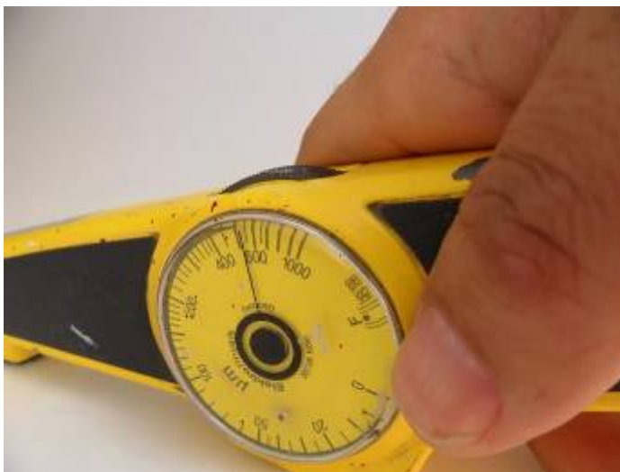
34. Epoxy resin paint thickness : 510µm
