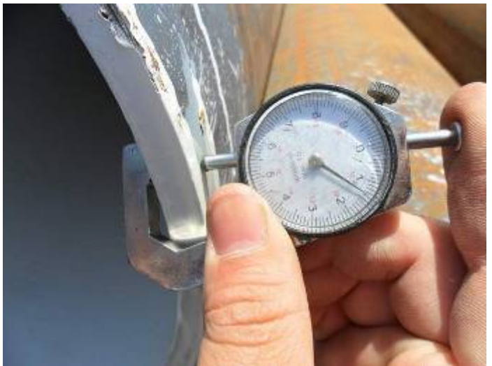
28. Wall thickness test : 11.3mm
