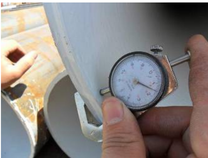
29. Wall thickness test :11.5mm
