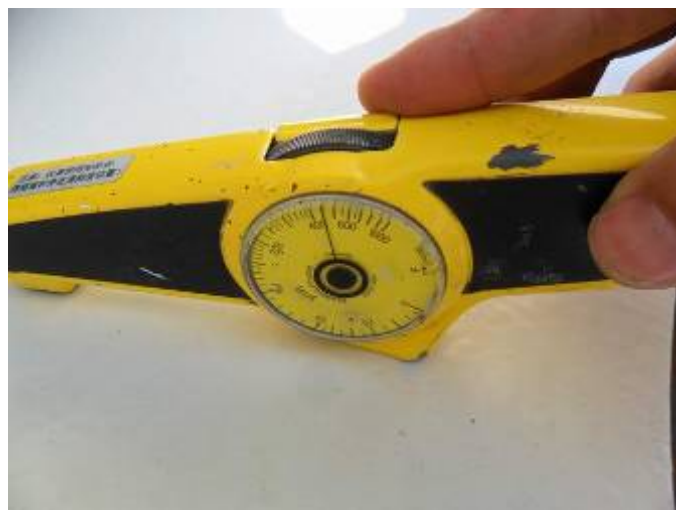
38. Epoxy resin paint thickness : 450µm
