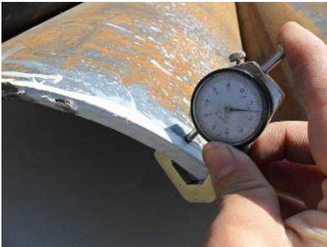
27. Wall thickness test :11.5mm
