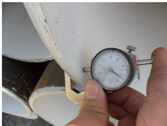
24. Wall thickness test :11.4mm
