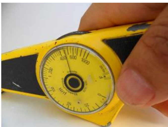
35. Epoxy resin paint thickness : 460µm
