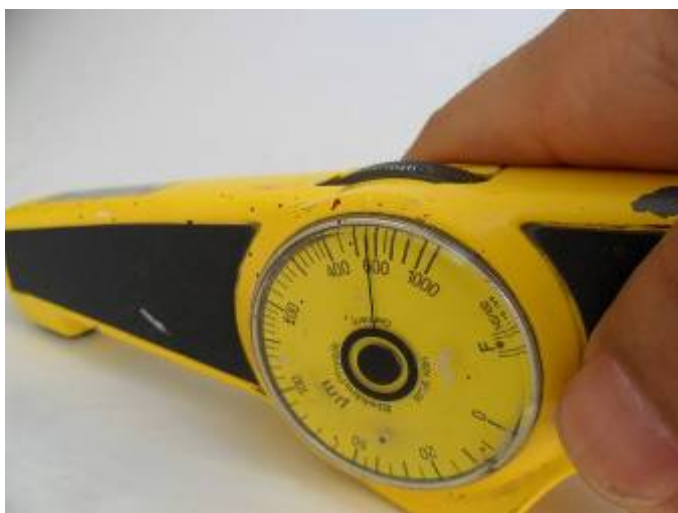
33. Epoxy resin paint thickness : 550µm
