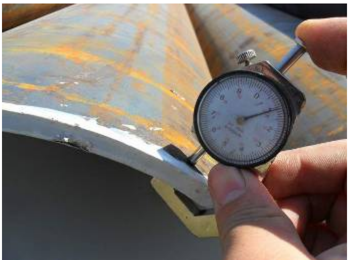
30. Wall thickness test :11.1mm
