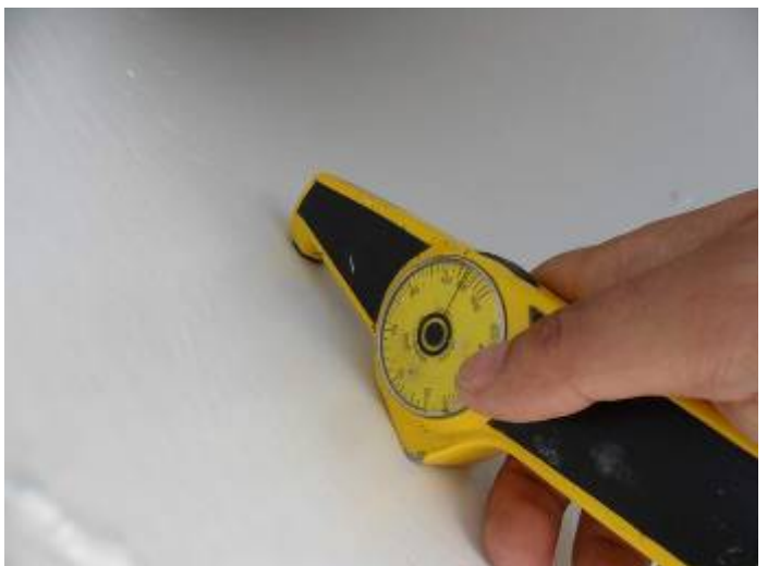
32. Epoxy resin paint thickness : 570μm
