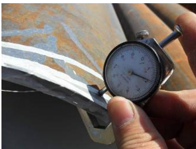
23. Wall thickness test :11.9mm
