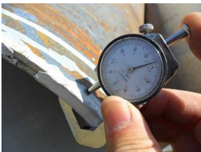
25. Wall thickness test :10.7mm
