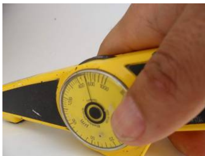
36. Epoxy resin paint thickness : 500µm
