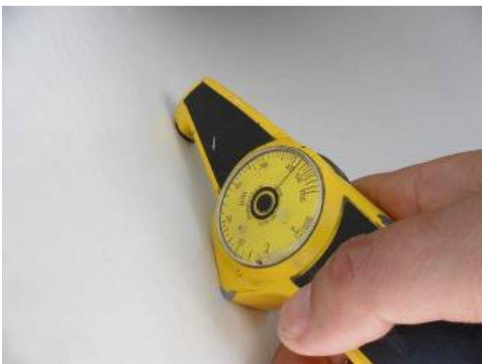
31. Epoxy resin paint thickness : 450μm
