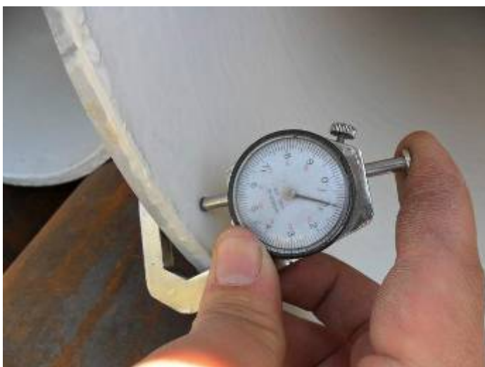
26. Wall thickness test :11mm
